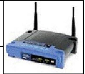
The two basic components in a wireless network are the access point and the wireless adapter that communicates with that access point. The access point serves as the base station for your network, emitting data signals that other computers on the network can receive and return. Each computer connected wirelessly to the network needs its own wireless adapter to connect to the base.
